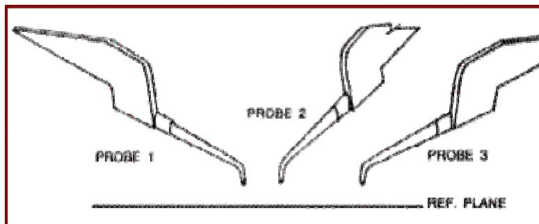
Figure 2 shows all three probe points to be on the same plane relative to each other but are not at the correct planarization depth.
